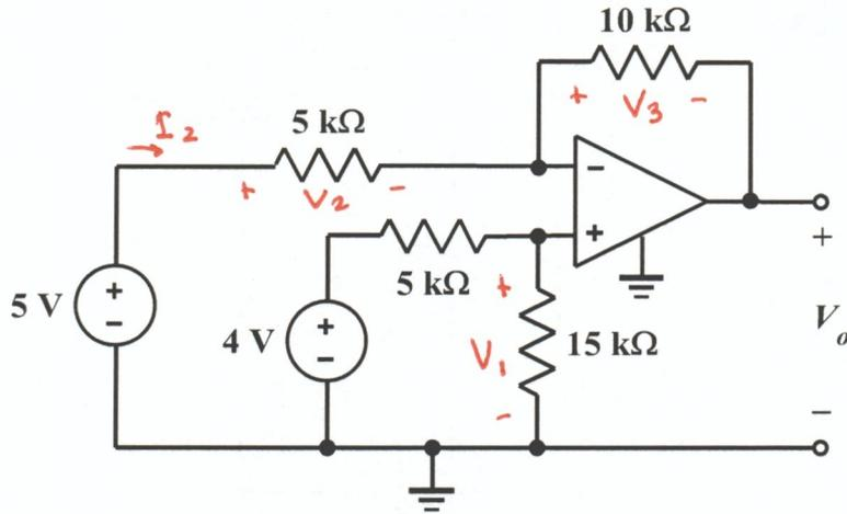
$$V_1 = \frac{15 \text{ k}\Omega}{5 \text{ k}\Omega + 15 \text{ k}\Omega} \cdot 4 \text{ V} = 3 \text{ V}$$
